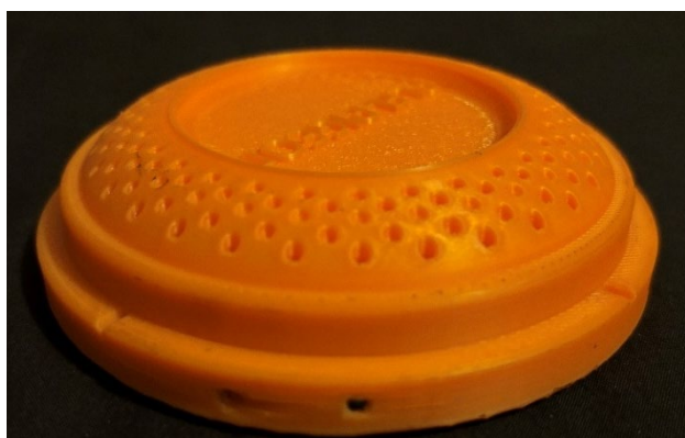
Figure 12 Pellet embedding on the optimized V12 with variable infill, showing reduced layer-line shearing compared to vertical 100% infill prints.
