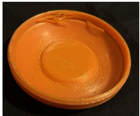
Figure 11 Most extensive damage observed on the variable-infill V12. Despite severe local deformation, the geometry remained intact and testing was successful.
