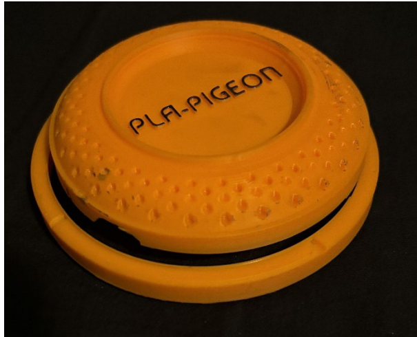
Figure 8 Weak point in V11 caused by sharp corners aligned with layer lines, resulting in catastrophic failure.
