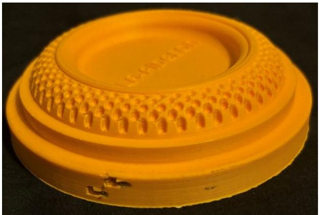
Figure 7 Vertical layer line shearing observed at impact points.
