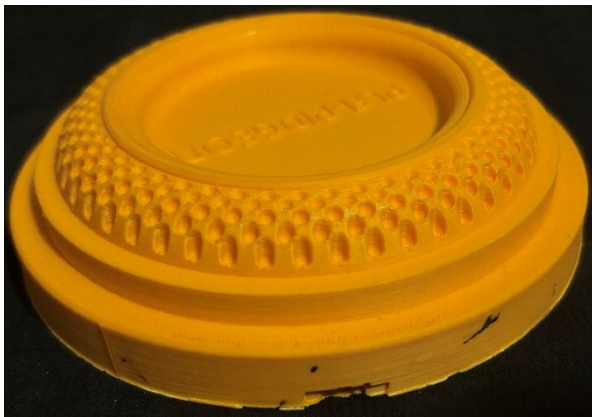
Figure 6 V4 tested at 100% infill. Impact occurred while flying from a standard sporting clay tower.
