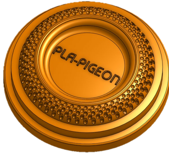
Figure 1 3D model of V4, the first PLA-Pigeon iteration tested for impact resistance. Results confirmed concept viability and demonstrated potential for further refinement.
