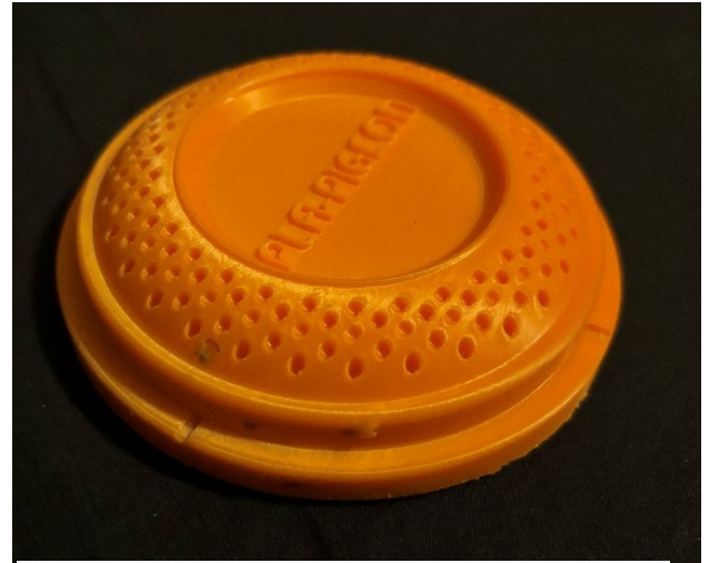
Figure 9 Post-test documentation of V12, 45° orientation. Target shows minimal deformation and no pellet embedding, demonstrating enhanced durability from angled layer orientation.
