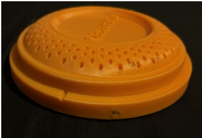
Figure 10 Pellet embedding on the 45° variant of V12, showing lack of layer-line shearing and a minimal entry wound.
