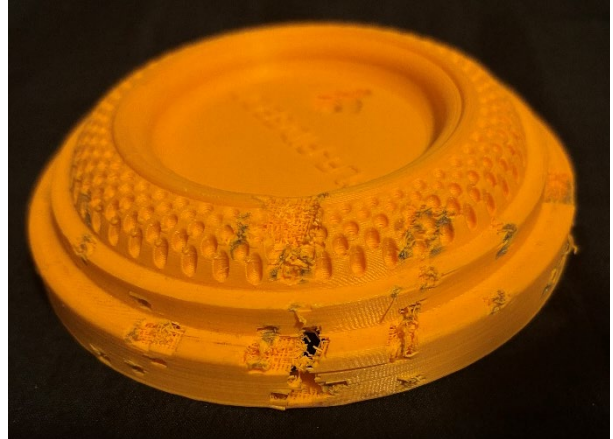
Figure 5 Despite increased surface damage, overall geometry remained consistent. Performance at > 100% infill showcased promise for improvements in durability.
